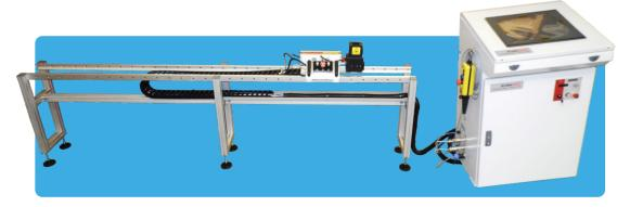
With this model, the laser head is mounted on a self-guided rail system, built to a customer's height and width specifications, usually to suit the dimensions and positioning of a tempering oven.
